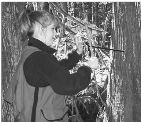
The past is revealed by coring into a tree: An Oregon City High School student uses an increment borer to look at recent growth rate of this western redcedar.
